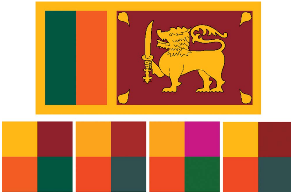
FIG. 1. Nearest neighbor colors to original (Left), in the W3C CSS Color Model definition for RGB (Middle Left), HSV (Middle Right) and CIELAB (Right).
